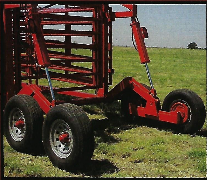
Walking I-bean carries the weight of the unit on rough ground. Electric brakes are on all four wheels.
