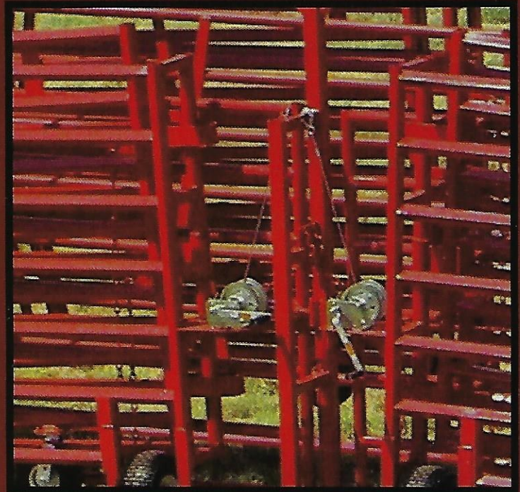
Two halves of the goose-neck enter lock together with TWO 1" bolts for transporting. This goose-neck hitch has an adjustment of 9".
